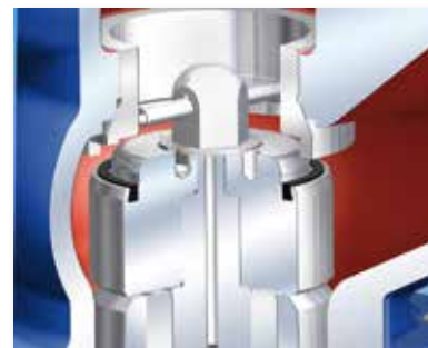
Plug with PTFE soft sealing (max. 200°C, only for standard Kvs-values)
