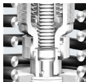
Sealing bellows as standard (PREDU® / PREDEX®)
