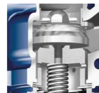
Thermal closing valve (for heating systems) closes when the temperature at the sensor rises
