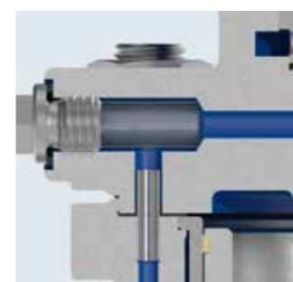
Safer due to additional integrated strainer
