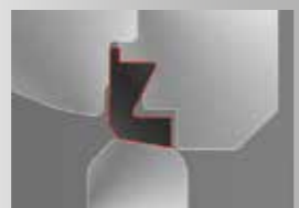
Tight sealing up to max. +180°C with PTFE sealing ring
